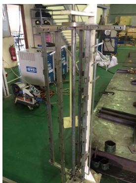
Painting JIG 塗装用治具
